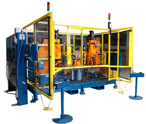
This custom dual workstation machine uses Tog-L-Loc® to assemble an automotive part.
