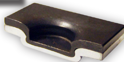
Cut away view of a completed Tog-L-Loc ® joint. Notice how the metal flow has formed an interlock.
